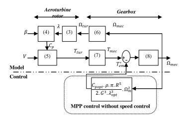
Fig. 6 Block diagram without speed control
