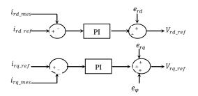
Fig. 10 Bloc diagram of rotor currents control
