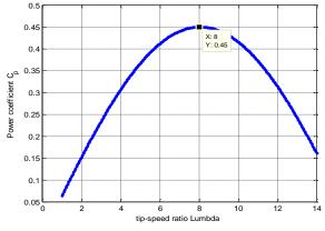
Fig. 7 Power coefficient versus tip speed ratio
