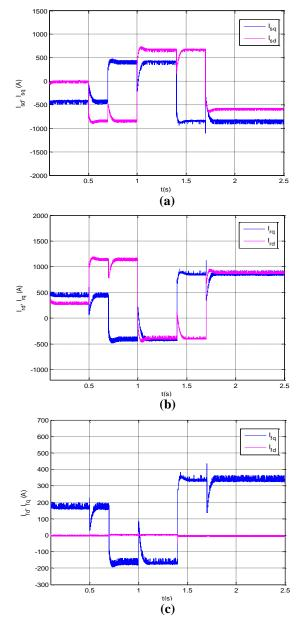
Fig. 15 Currents d-q axis in super-synchronous mode
