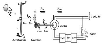
Fig. 1 Schematic diagram of DFIG wind turbine
