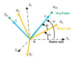
Fig. 5 Orientation of the d-q frame
