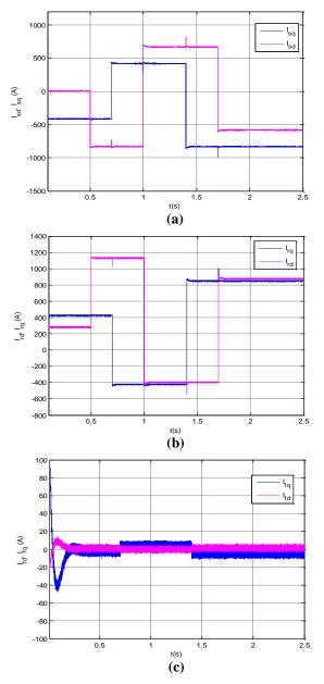
Fig. 14 Currents d-q axis in sub-synchronous mode
